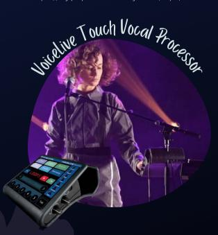
The VoiceLive Touch is a vocal effects processor, which is a digital device that allows vocalists to add effects to their voice as they are performing. There is a range of effects such as, echo, voice doubling, and reverb. The device connects through XLR cables to take input through the microphone and runs it through the processor allowing the finished product to be relayed through the speakers.
